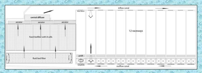
Central diffuser provides discharge 312 l/s, maximal opening of the flow block in first Raceway cause inflow 78 l/s, flow velocity and discharge decreases along inflow canal
