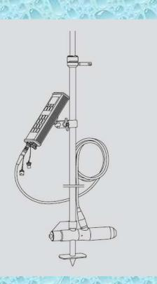
Used for discharge measurements in open channels according to the EN ISO 748
